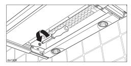
Note for dismantling the cooker hood: Undoing the screws on the left and right inside the housing releases the brackets, allowing the appliance to be removed from the unit
